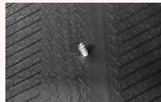
Foreign object detection inside tire
